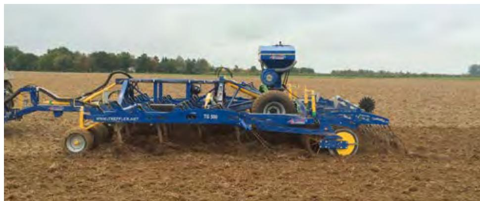
tractor is not carrying any extra load, the tractor can be run with extremely low tire pressure. Combining precision depth control with 6 mm thick self-sharpening duckfoot tines positioned at a small angle to the ground makes this machine particularly suitable for soil preparation in spring.
