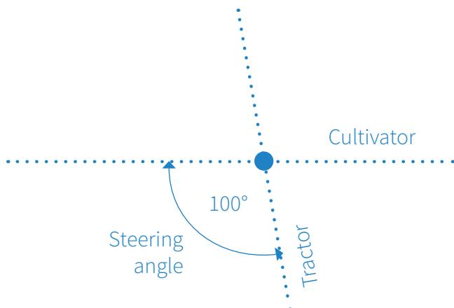
As the coupling point is attached to the lower linkage of the tractor, and the pivot joint of the cultivator can swivel without restriction in both horizontal and vertical direction, steering angles of up to 100 degrees can be achieved, depending on the tractor model and tires.
