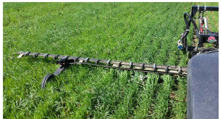
Mechanical weed control with hydraulically height-adjustable feeler wheel
